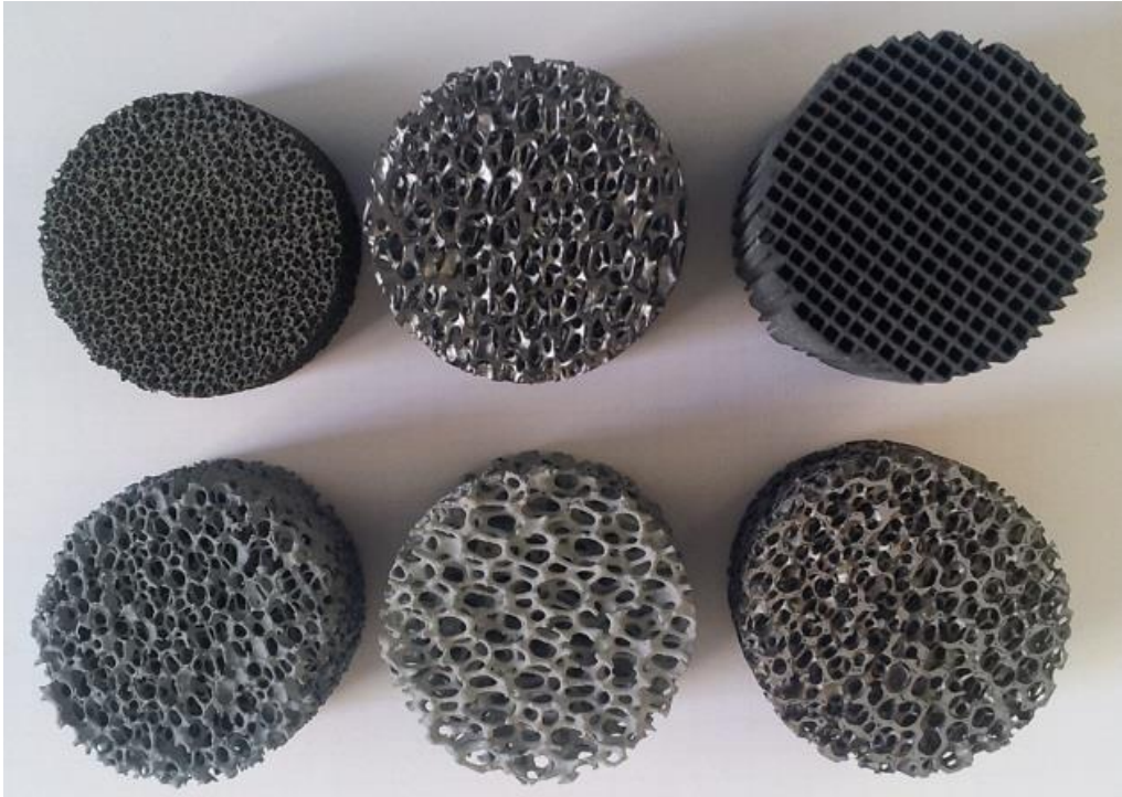
Fig.7: First line: \alpha -SiC, Si-SiC, and SiC honeycombs. Second line: SiC+Al 2 O 3 , SiC+SiO 2 +Al 2 O 3 , ZrB 2 .
