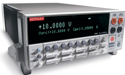
Figure II.7 – Photo d'un Keithley 2400 source-meter.
