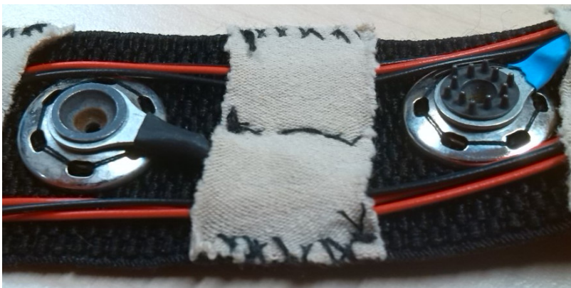
Figure C.5 – Close-up of the attach system. EL120 electrodes are snapped to a size 10 Dritz and contact with the cable leads is made through crimp rings. Middle: a man that knows his sewing. Or not.
