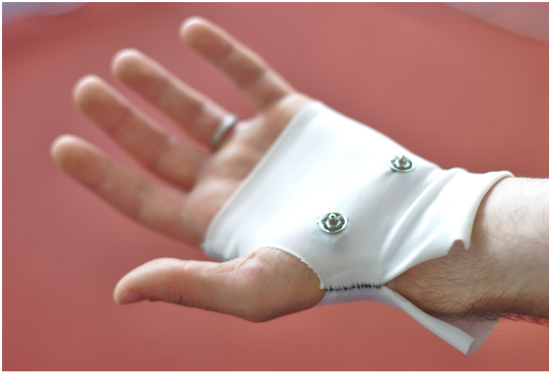
Figure 11.5 – Wearables: fingerless glove measuring EDA.
