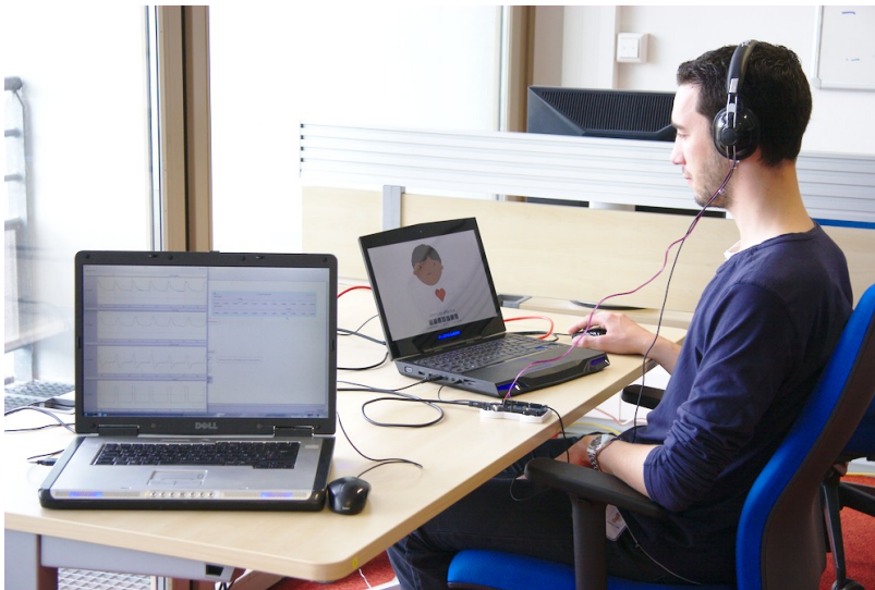
Figure 8.5 – Our experimental setup. A BVP sensor connects participant's earlobe to the first laptop, where the human-agent interaction takes place. Participant is wearing a headset to listen to the speech synthesis. A second laptop is used by the experimenter to monitor heartbeats detection.
