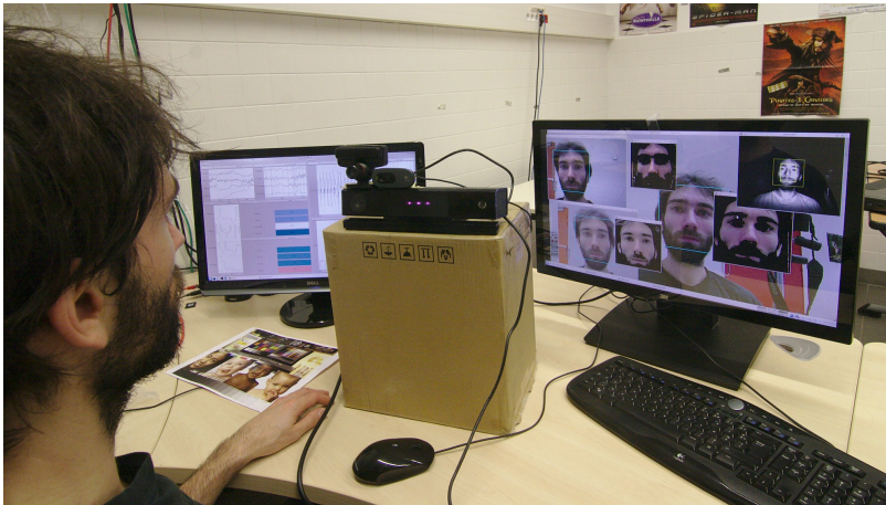
Figure D.2 – Experimental setup used during the experiment. Altogether with recordings from ECG electrodes placed on the torso, 3 webcams were recording subtle changes in skin color.
