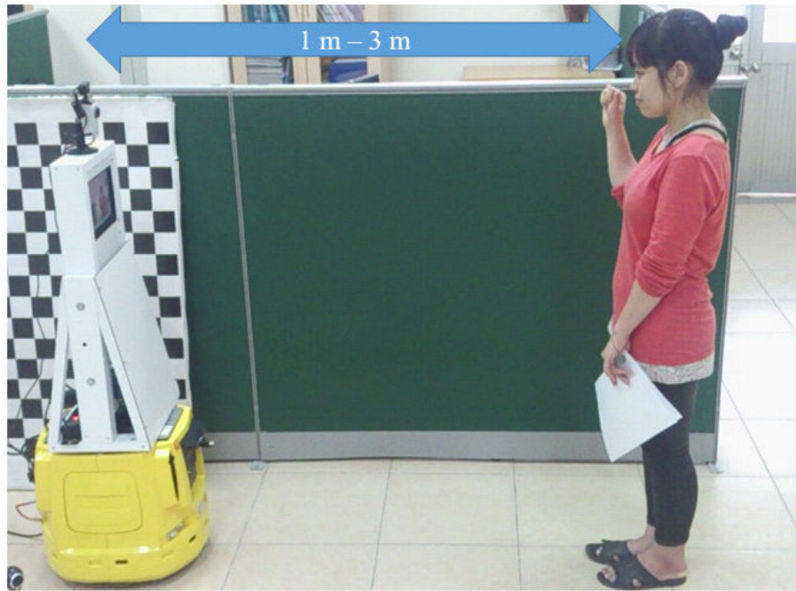
Figure 3.22 – The illustration of the setup of capturing dataset.
