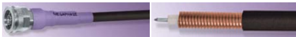
Figure 3.8: Structure of coaxial cable: inner conductor–solid Ag-plated Cu, dielectric–PTFE, and outer conductor–GrooveTube® Cu
