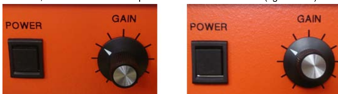
Figure 4.20: Different point views of amplifier control knob which may introduce power level adjustment error.
