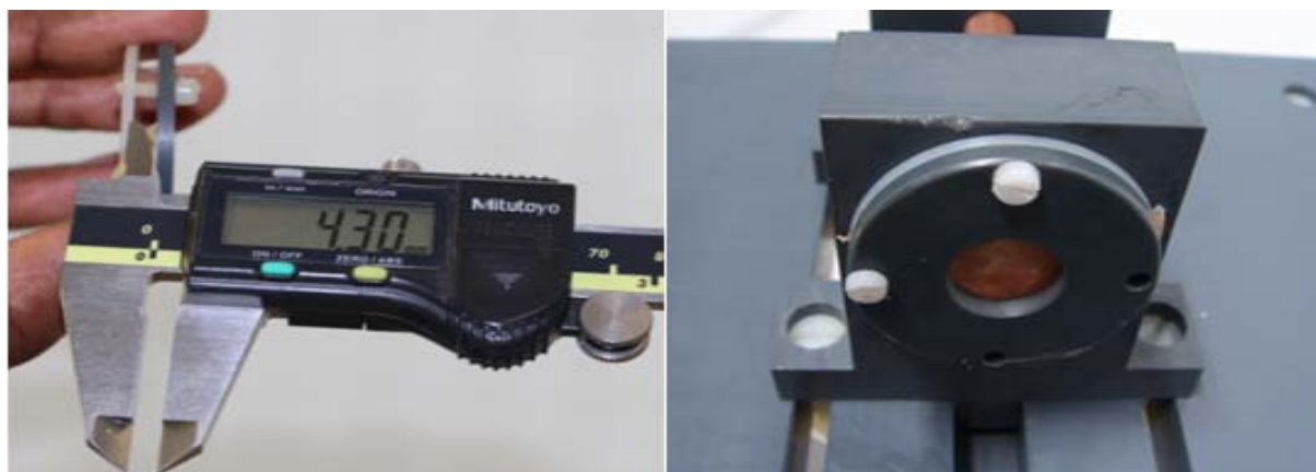
Figure 3.6: Maximum thickness of biological sample can be 4.3mm corresponding to the length of the sample holders fixture screws
