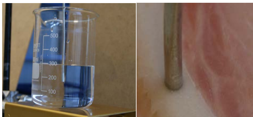
Figure 2.11: Coaxial probe's extremity should contact well with the measured materials
