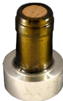
Figure III.3.5: Bottleneck inserted in a metal ring for oxygen transfer measurements
