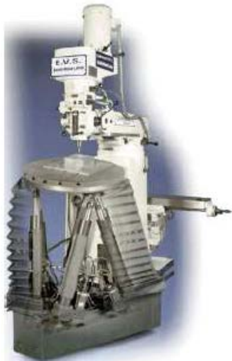
Figure 1.20 : La machine Hexabot
