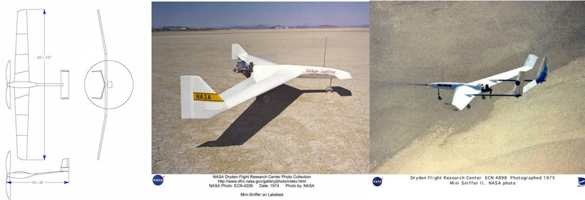
Figure 4. Three of the configurations explored in this study: Left, wing and 2 tails design; center, wing and canard design; right, swept wing and 2 tails design.
