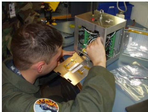
Figure 13. USAF Academy Cadet Performing Final Assembly of a Revision A EyasSAT Spring 2004
