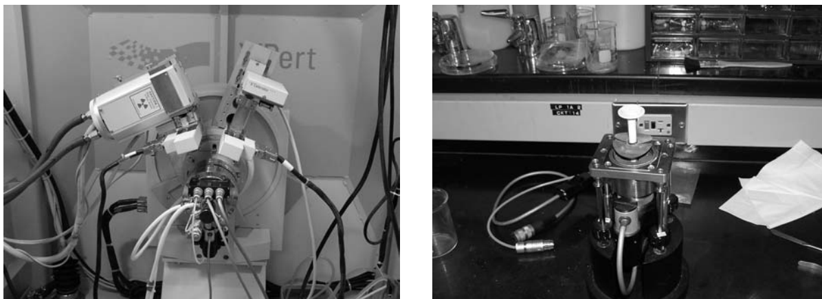
Figure 2.1: Left; X'Celerator "Real-Time Multiple Strip" detector and the Anton-Paar HTK 1200 high-temperature stage, Right; Sample holder.
