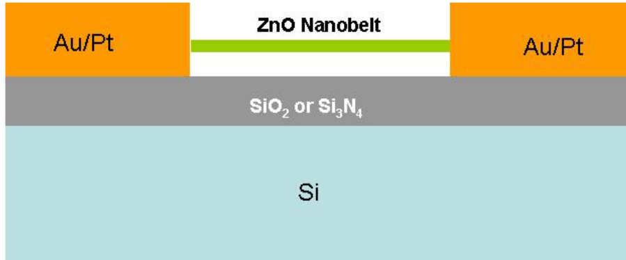
Figure 2.6 A simplified cross-sectional schematic of the device structure.
