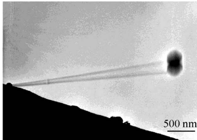
Figure 6.8 Measurement of the work function of an attached carbon particle on the tip of a ZnO nanobelt at f = 0.349 MHz and V_{ac} = 9.0 V.
