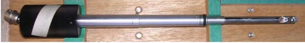
Figure 6.2 A top view of a home-made sample holder for in-situ TEM measurement.
