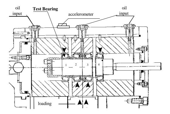
Figure 15: Schematic of Test Housing
