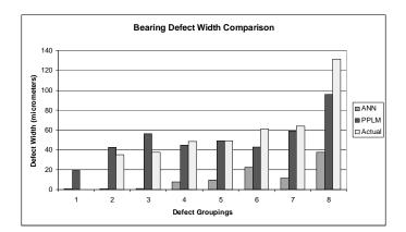
Figure 16: Bearing Defect Width: Predictions vs. Actuals
