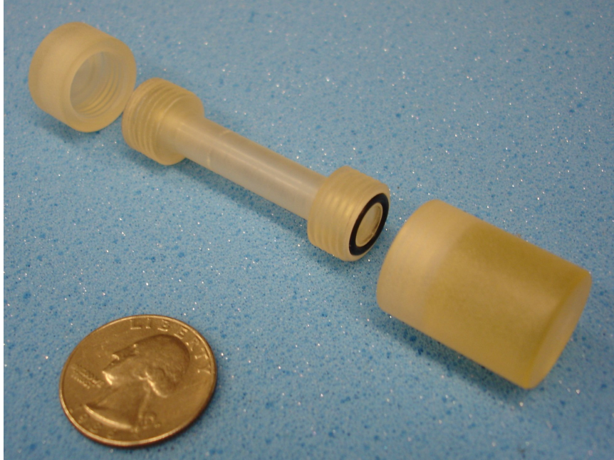
Figure 6-3. VivaCT sample holder for static and rocker control constructs. O-ring seals on either end prevent media leaks and maintain sterility in the VivaCT. Three constructs can be placed in the holder at one time to minimize overall scan time.
