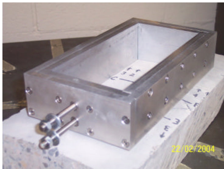
Figure 3.10 Shear Box on Top of the Pipe Coupon
