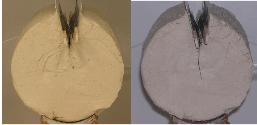
(a) Ice lens evolution when subjected to tension
