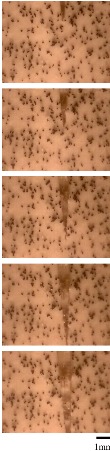
Figure 5.7 Ice lens growth with time. A thin opening at the lens tip is observed prior to lens growth.
