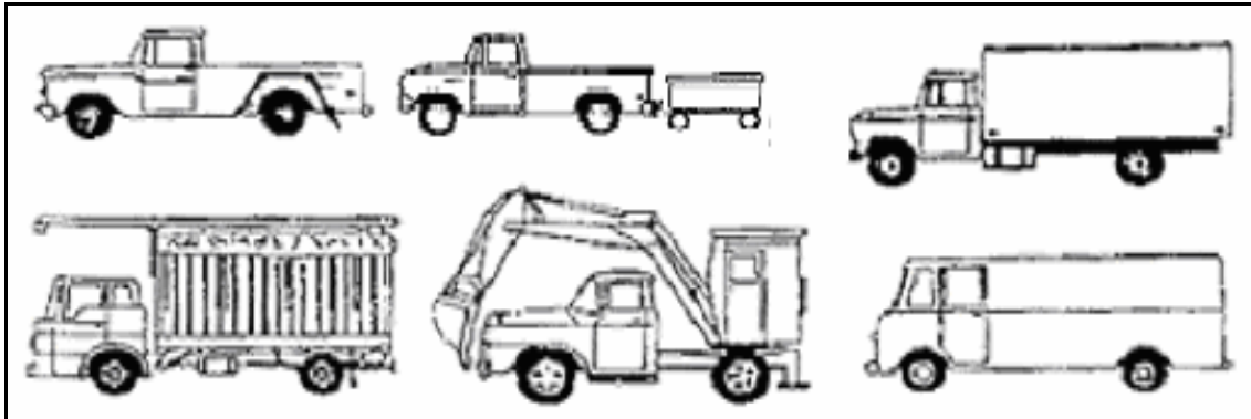
Figure 6.1: Class X1: 2-Axle HDVs, 8,501 to 33,000lbs of GVWRs
