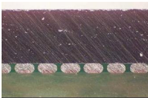
Figure 1.4 Excellent Soldering Achieved Using Nano-filled No Flow Underfill [Prabhakumar, 2004]
