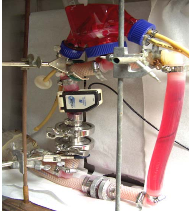
Figure 4.6: Picture of the organ culture system with porcine aortic valve cultured in the system.
