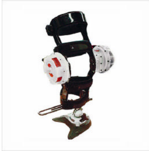
Figure 9 – Knee brace with electrorheological fluid www.robots.neu.edu
