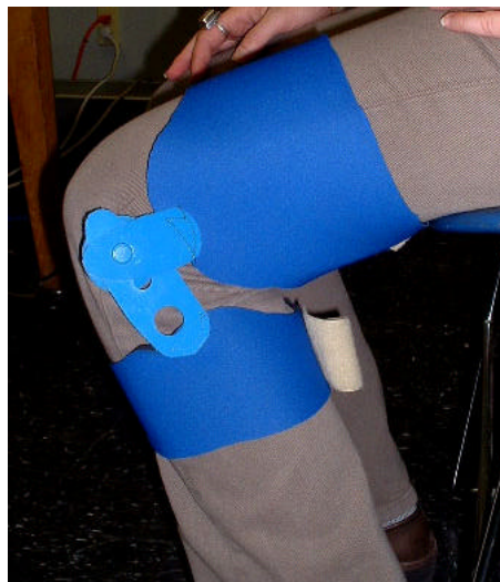
Figure 24 - Neoprene prototype with Hytrel
