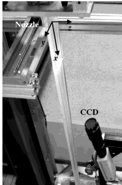
Fig. 3. Photograph showing the liquid sheet illuminated by the laser light sheet imaged obliquely from below by CCD camera.
