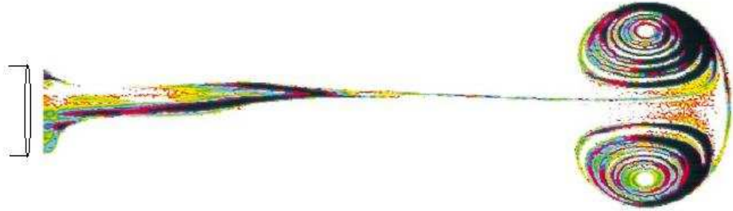
Figure 51: Experimental visualization of a vortex ring created by the impulsive injection of water from a tube. Taken from [16].
