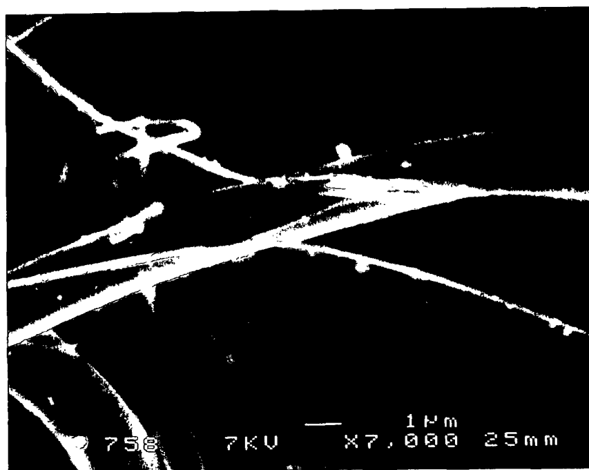
Figure 26. SEM photomicrograph showing fume on BGF filter fibers. Conditions given in Fig. 25. Magnification 7,000 ×.
