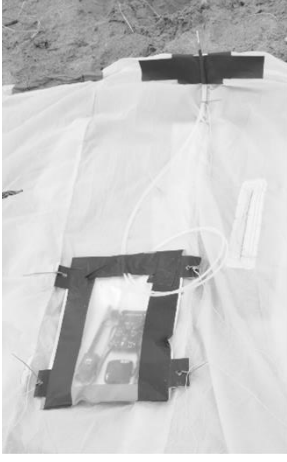
Figure 8: Pixhawk and pitot tube mounted in kite bridle
