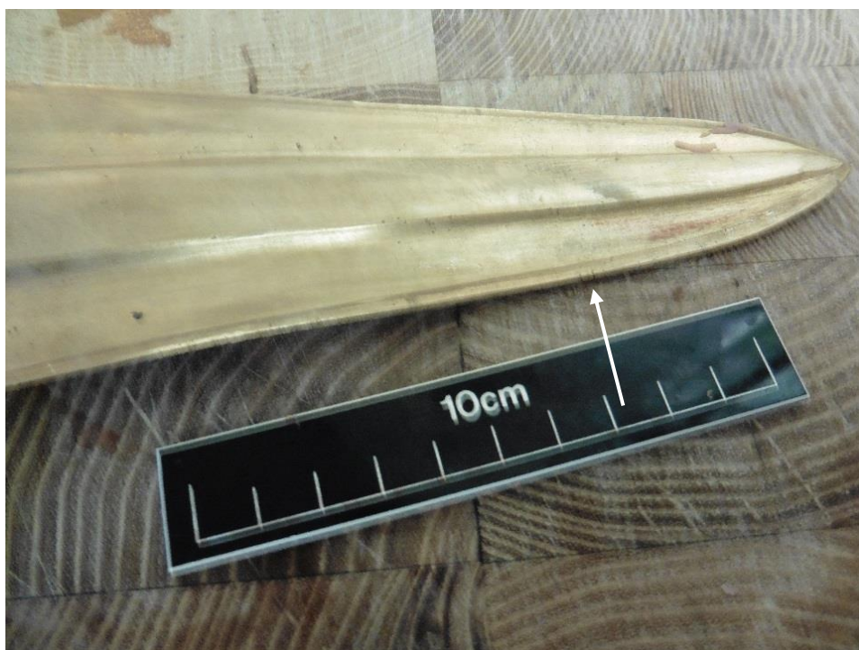
Figure 7.6 – The small U-shaped notching edge damage caused by the replica blade snagging on the scapula.
