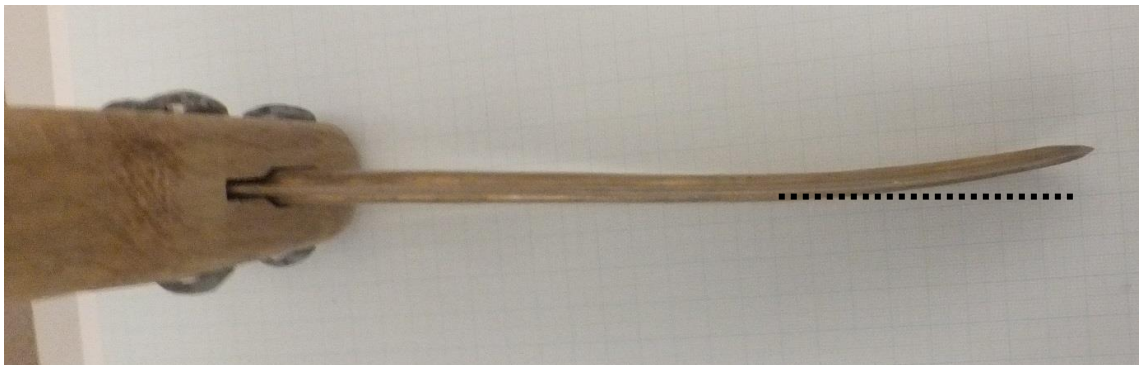
Figure 6.20 – The 12° bending deformation of the first replica halberd after the second blow, with the original straight line of the blade indicated by the black dotted line.
