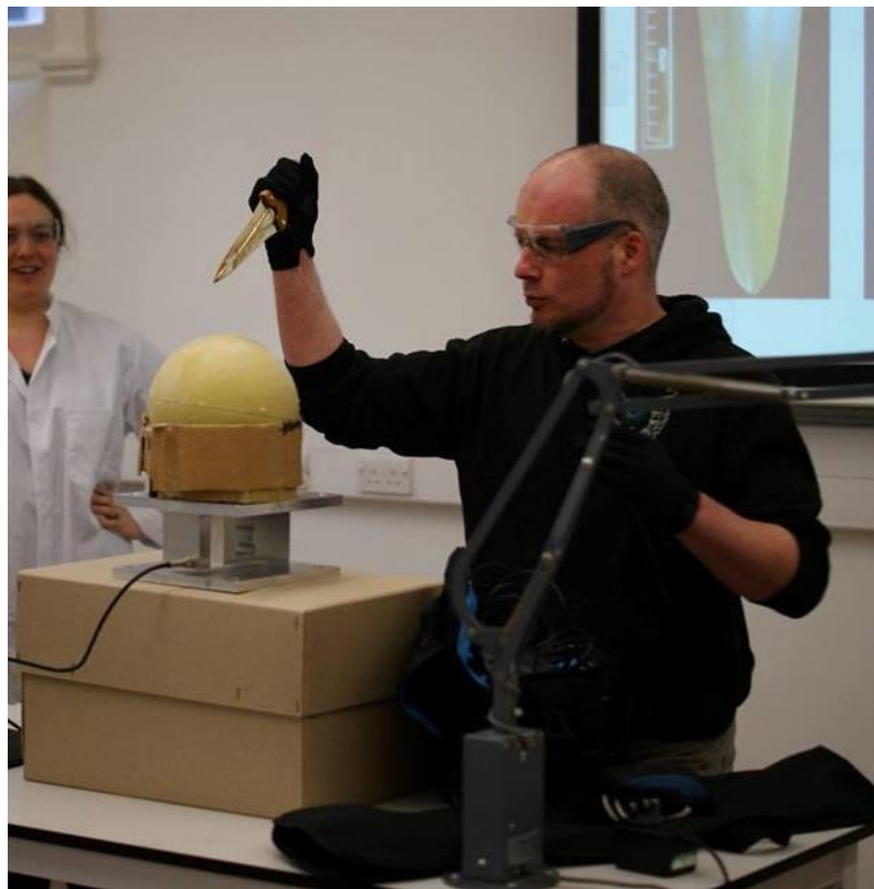
Figure 3.10 – The strong sweeping overarm blow being delivered. The Synbone™ sphere is clearly visible, anchored in a circular cardboard sheath and sitting atop the force meter.
