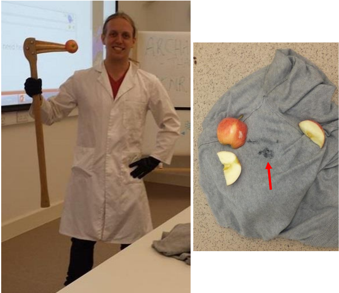
Figure 6.17 – The wielder’s target practice using the replica halberd. Left: the results of the first on-target blow. Right: the almost inevitable result of the second on-target blow. The foam pad was also punctured (red arrow); this indicated that the halberd’s penetrative power was greater than initially expected.
