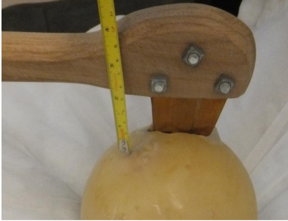
Figure 6.23 – The clean puncture made by the first blow.
