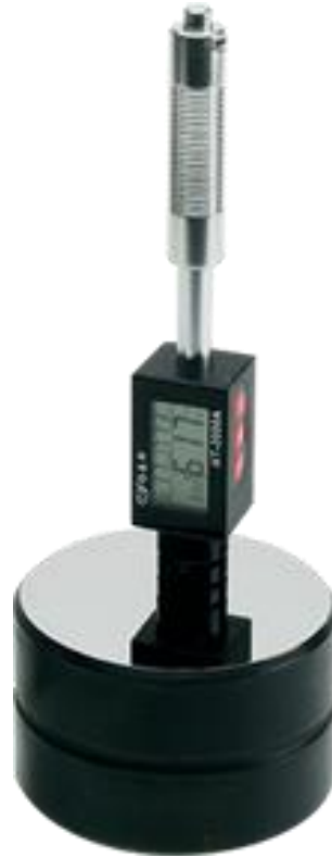
Figure 3.9 – The portable hardness tester. http://grhardnesstester.com/
