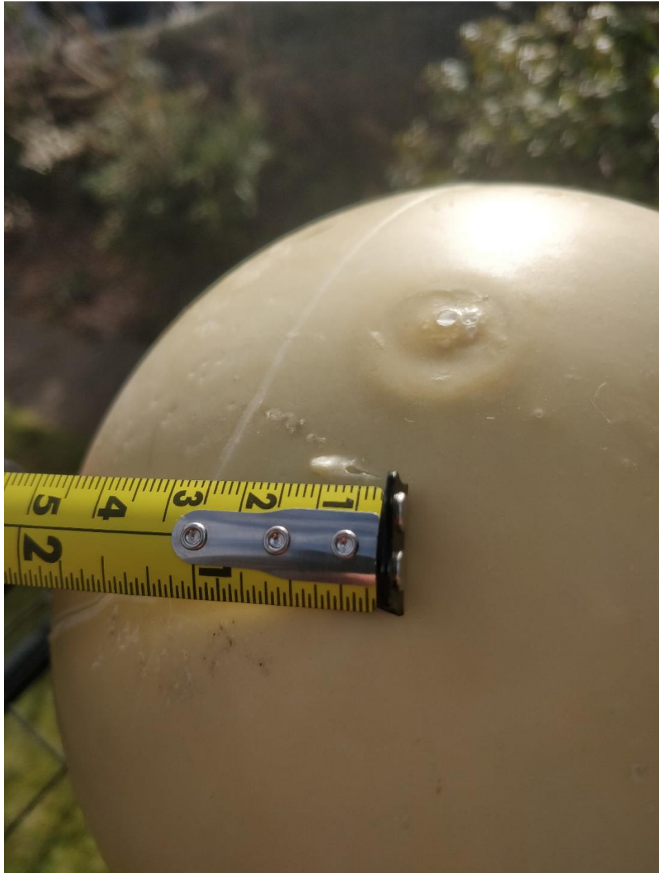
Figure 6.8.4. Damage inflicted by the second blow with no relative height difference. The rubber skin has been pierced, and the miniscule damage to the underlying bone is visible on the right of the cut.
