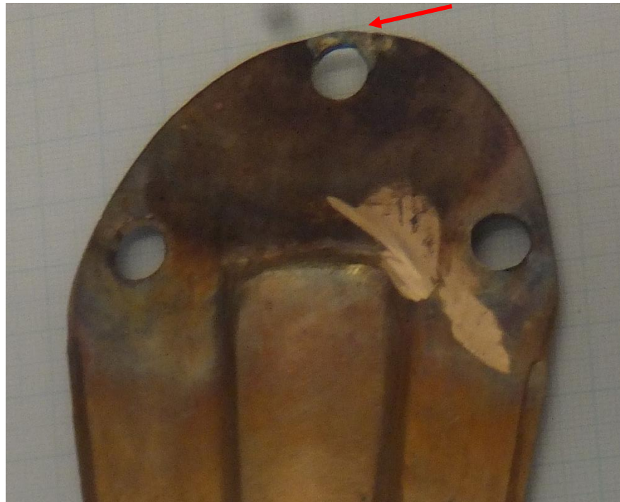
Figure 6.27 – The second halberd blade after all four blows. The narrow, deformed metal bridge on the central rivet hole is indicated by a red arrow. The superficial discolouration of the bronze is due to the natural oils and resin in the oak handle.
