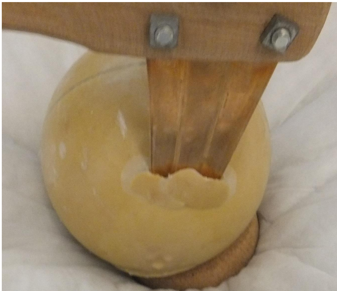
Figure 6.25 – Puncture and flake damage from the third blow using the second halberd.
