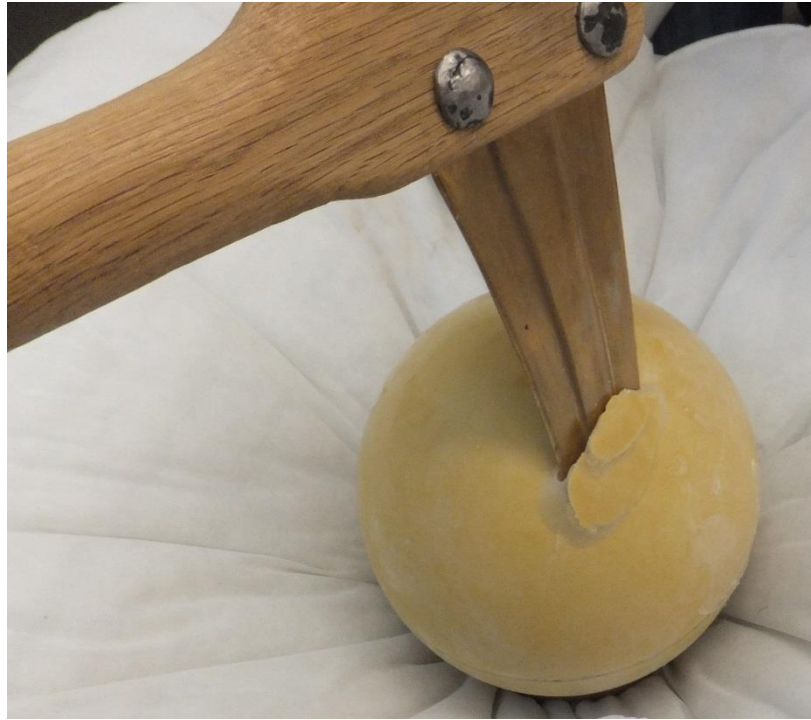
Figure 6.18 – The first blow using the riveted halberd on the first Synbone™ sphere. The large detached flake is clear, with the smaller flake fragmenting from its uppermost edge.
