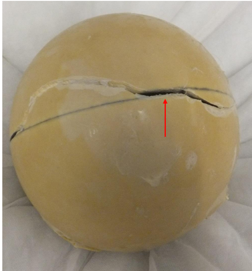
Figure 6.26 – The lateral fracture resulting from the fourth blow with the second halberd. The red arrow shows the entry point of the blade. The fracture can be seen curving sinuously across the dark blue suture line.
