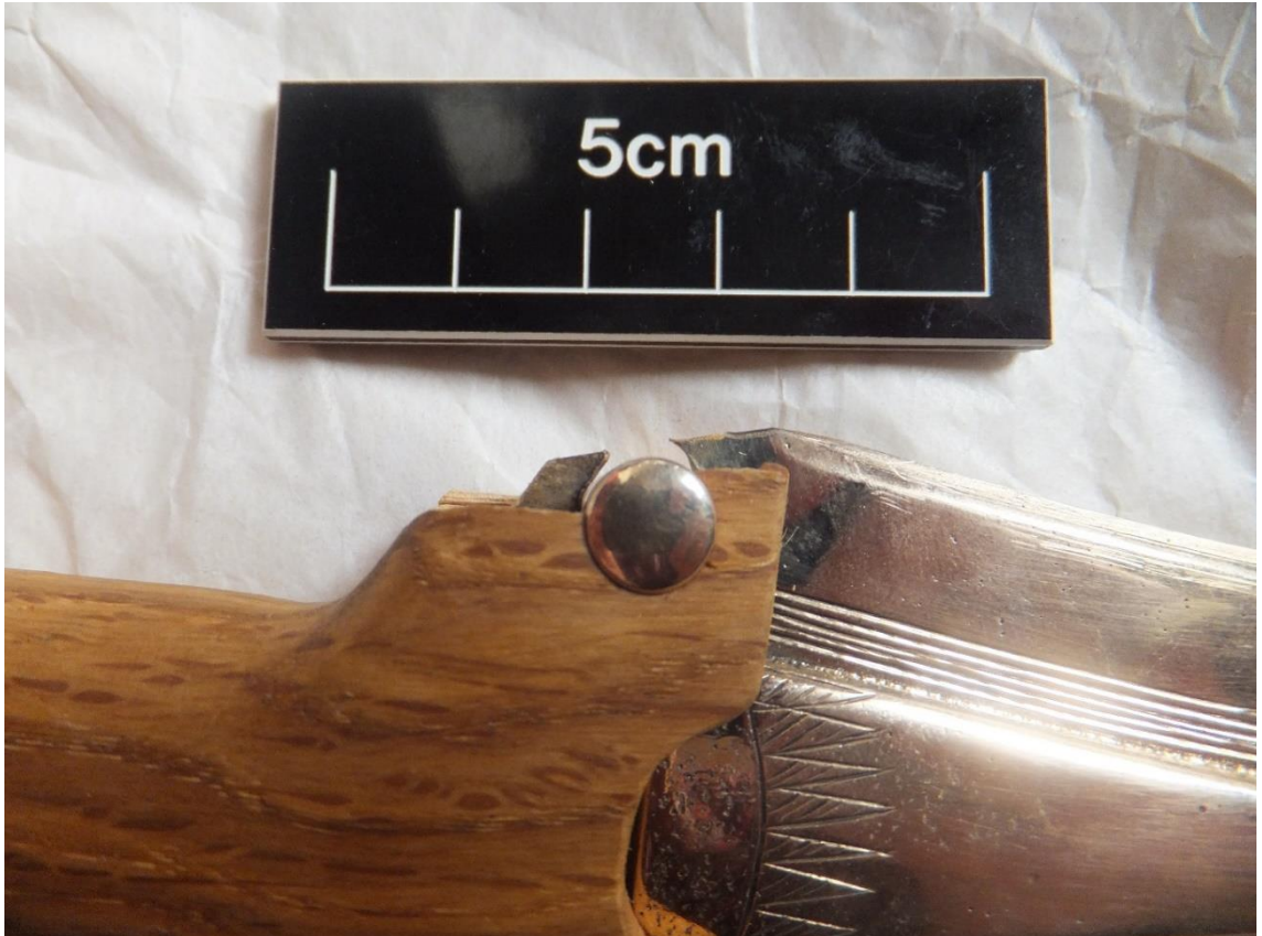
Figure 3.12 – Damage to the rivet and hilt from the connecting overarm blow. The clean linear shear was a thoroughly unexpected result of the trial. ©Perth Museum and Art Gallery, Perth and Kinross, Scotland.
