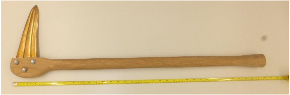
Figure 6.13 –Handle 1, made by Neil Burrige, after hafting the blade. The nuts and bolts used to affix the blade to the handle can be seen.
