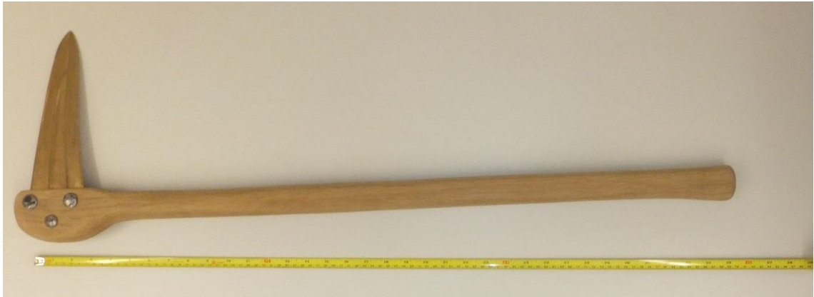
Figure 6.15 – The second halberd handle (Handle 2) with riveted blade (metre scale bar).
