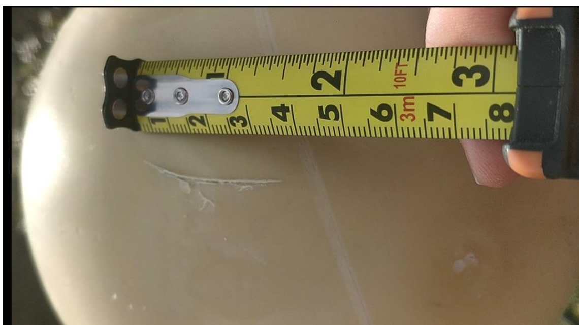
Figure 6.8.9. The third and final blow. This blow caused no damage to the skeletal material but did slice the rubber skin in a 35mm long scratch.
