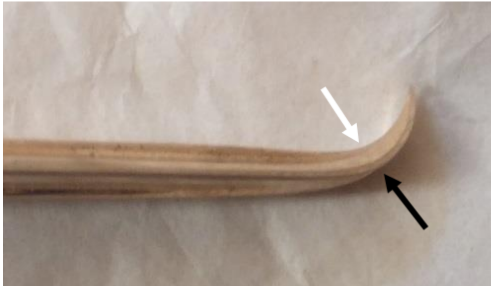
Figure 8.10 – The bent tip of the replica dirk following the Synbone™ experiments described in Section 3.4. The white arrow indicates the ‘inner face’ of the curve, which when hammered flat, produces smaller and/or fewer stretch tears. The black arrow indicates the ‘outer face’ of the curve, which produces larger and/or more stretch tears immediately the bending deformation occurs. © Perth Museum and Art Gallery, annotations author’s own.
