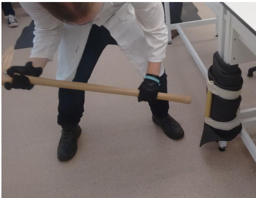
Figure 6.32 – The first attempt at a blunt-force trauma test; the blade can be seen close to the wielder’s shoulder and elbow, which caused some safety concerns. Image courtesy of Prof. Ian Ralston.
