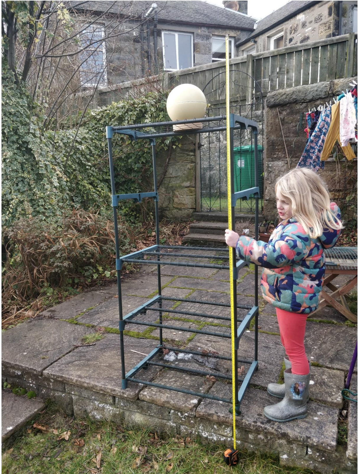
Figure 6.8.1. The Synbone sphere on the frame, with a 2m scale for reference. Measuring from the flagstones, the sphere is 1.6m (5ft 3in) from the ground; stepping down and measuring from the grass, the sphere is 1.75m (5ft 9in) from the ground.
