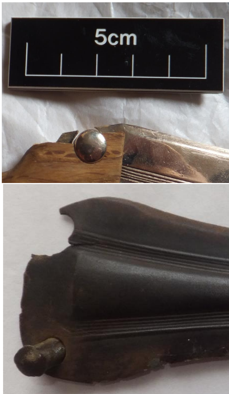
Figure 3.23 – The damage to the replica dirk as a result of the haft blow (top) and the single area of damage to the prehistoric dirk (bottom). © Perth Museum and Art Gallery, Perth and Kinross, Scotland
