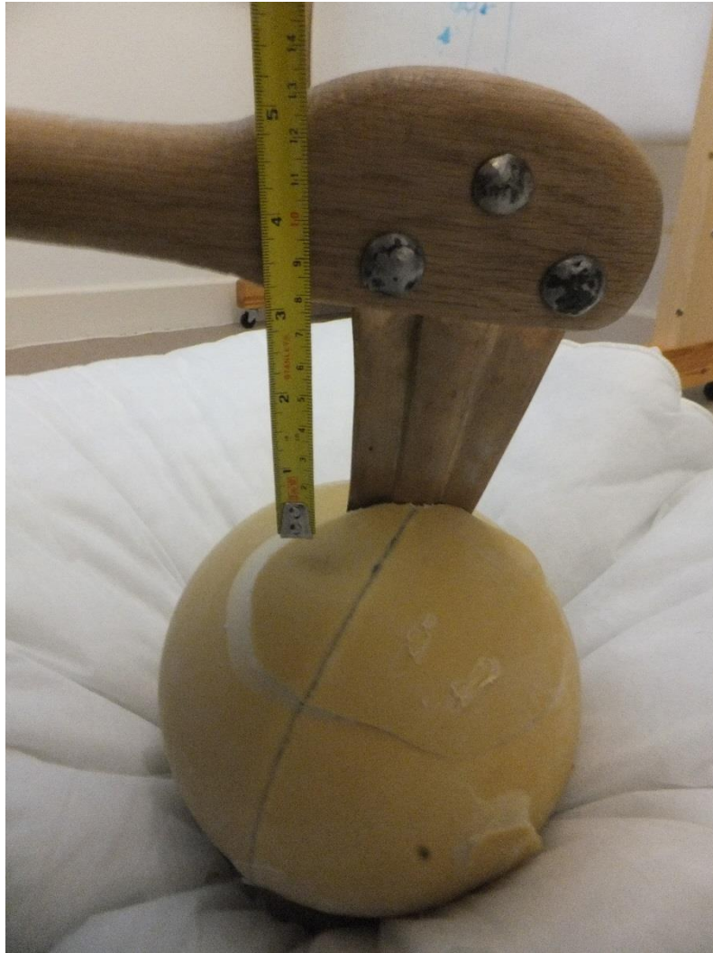
Figure 6.22 – The third blow with the first halberd. The large flake can clearly be seen to have completely detached from the sphere, and the thin rubber skin has stretched to accommodate the movement.
