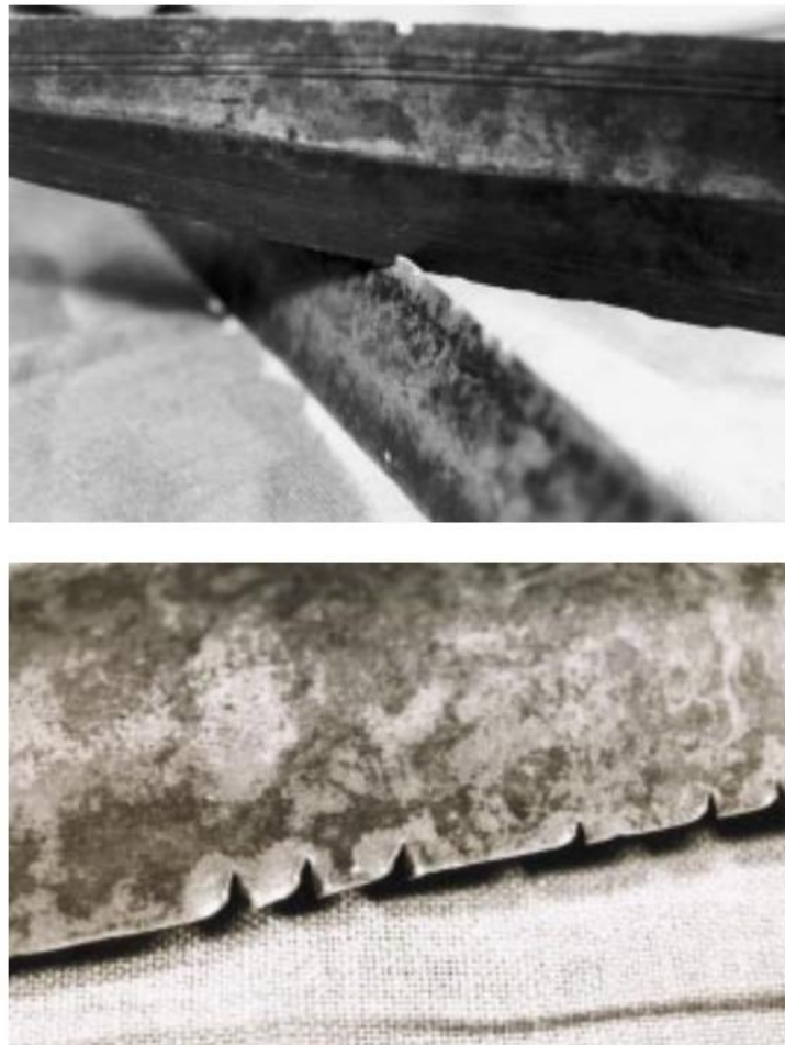
Figure 3.3 – Examples of the damage inflicted to the blades as part of the unspecified trials undertaken by Professor Kristiansen . The lack of scale bars, labelling and colour in the images throughout the paper seriously limits the utility of the study. Kristiansen (2002:325)
