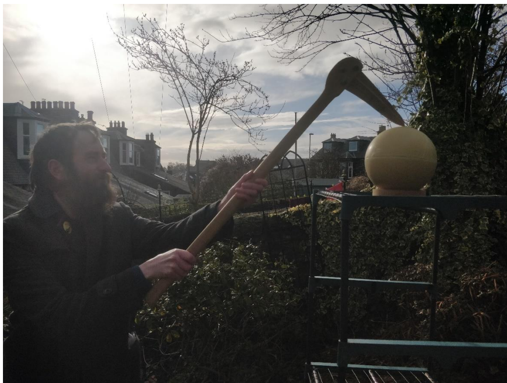
Figure 6.8.3. The second blow with no relative height difference. Note the acute angle of impact between the blade and sphere due to the higher target.
