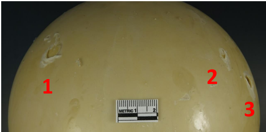
Figure 3.14 – The Synbone™ sphere showing all inflicted damage from the sharp and blunt force blows. Left to right: 1 - the ripped ‘skin’ from the third blow, the blunt force impact using the butt of the hilt; 2- the ripped ‘skin’ from the first blow, the first sharp force impact which glanced off the side of the sphere; 3 - the pierce and flake damage from the second, the connecting sharp force trauma impact which resulted in significant damage to the replica dirk. © M Downing 2015.
