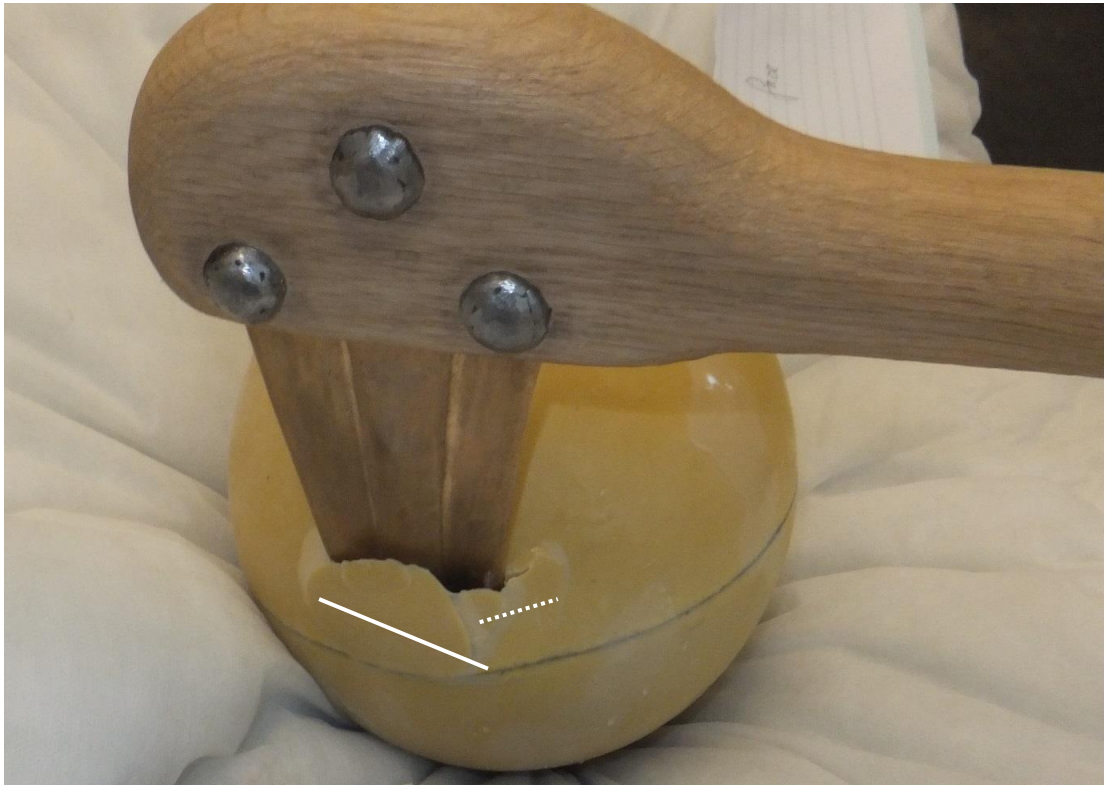
Figure 6.19 – Damage inflicted by the second blow. The solid white line indicates the extent of the flake, caused by the punching impact of the tip. The dotted white line indicates the jagged linear incision, caused by the widening of the blade as the weapon continues downwards into the sphere.
