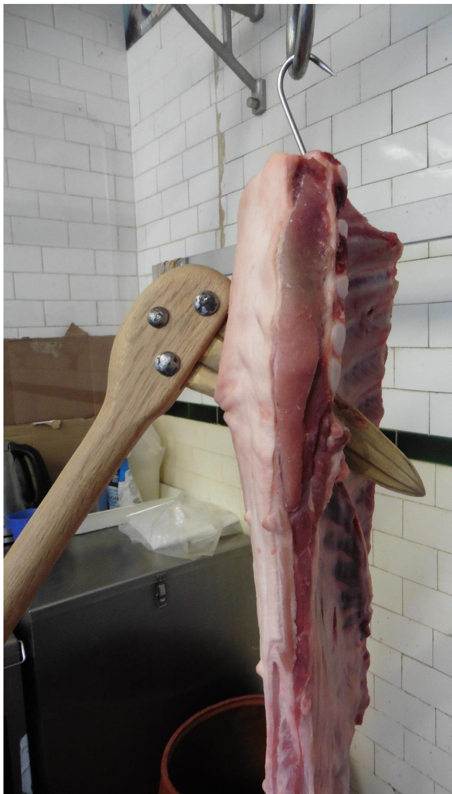
Figure 7.17 – The seventh blow. The angle of impact is visibly more inclined than previous blows, this is a product of the trajectory of the halberd blade due to the taller wielder.
