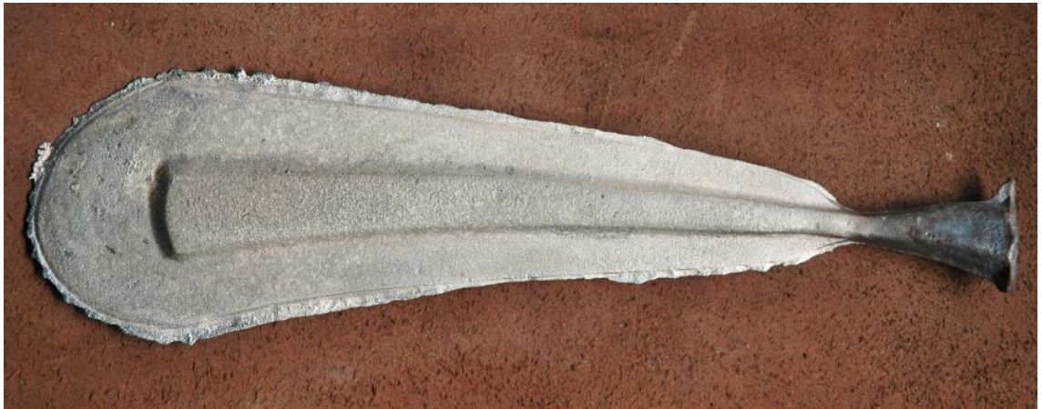
Figure 6.6 – The test cast. The rough edges are clear, as is the excess flange at the tip, where the molten bronze was poured into the mould.
