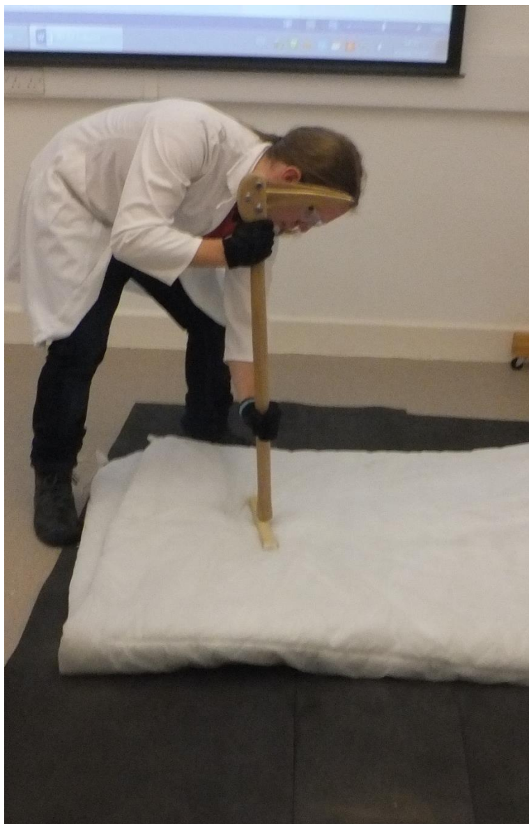
Figure 6.33 – The second experimental blunt-force trauma setup, with the long Synbone™ tube flat on the floor padding, and the connecting forceful vertical clubbing blow.
