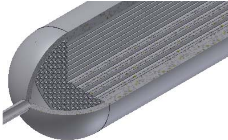
Figure 5-6: 316 Stainless Steel Reservoir (Turbine simulator)
