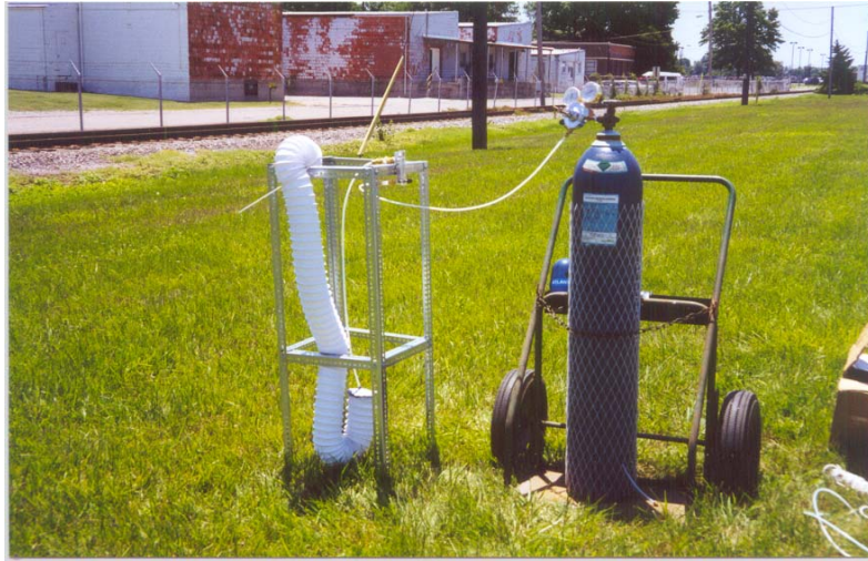
Figure 3-2. SF 6 release unit
