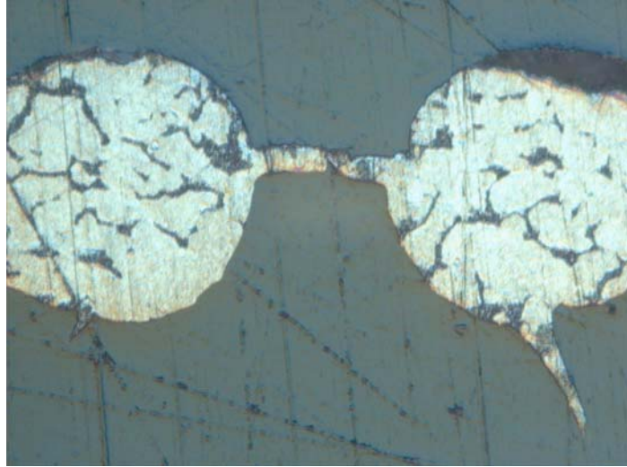
Figure 5-8 Solder Extrusion Into an Underfill Crack Causing a Short
