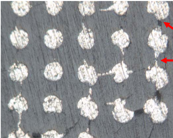
Figure 5-18 Material B, 3800 AATC cycles, extensive solder shorting
