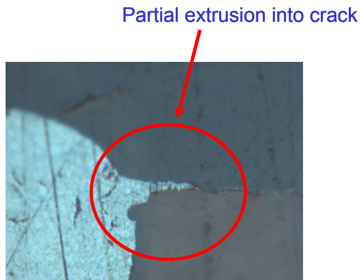
Figure 5-13 Material A, Partial Solder Extrusion Into a Crack, Part Removed From Test at 3500 Cycles
