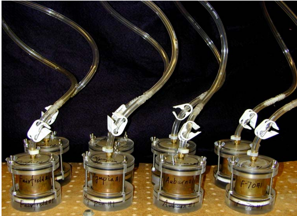
Figure 4-1. Tempe cells used to measure water retention characteristics (moisture release curves) of the soil samples
