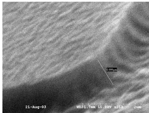
Figure 68. SEM picture showing etched shape by standard aluminum RIE process
