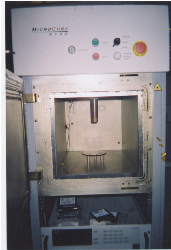
Figure 2-5 MicroCure 2100 Variable Frequency Microwave furnace used in research.
