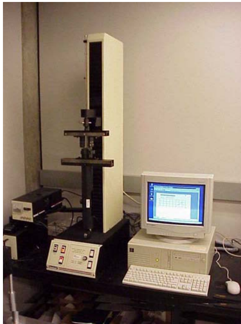
Figure 14. Computer controlled load frame used for flexural bend testing and interfacial fracture toughness testing
