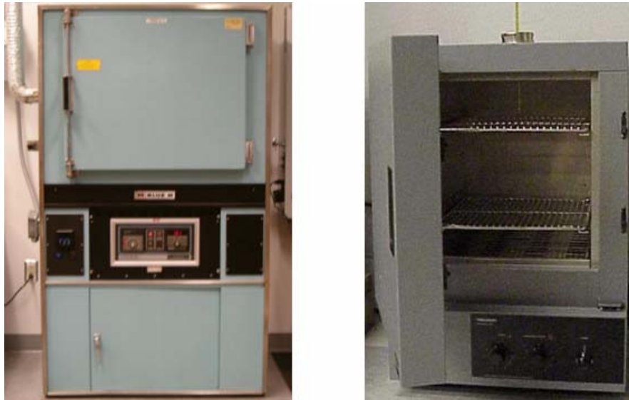
Figure 16. Convection ovens used for curing underfill resins and thermal aging test specimens
