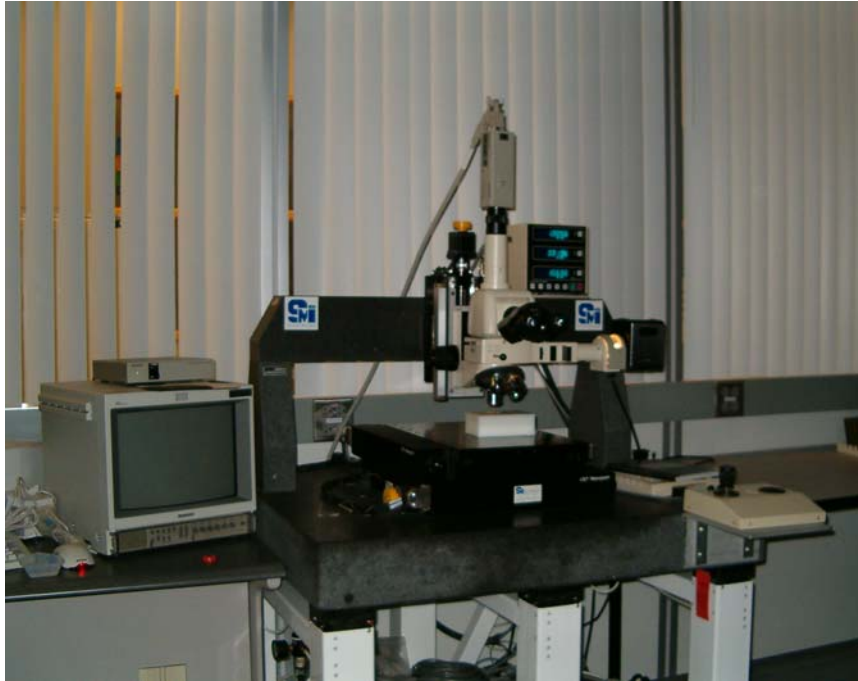
Figure 18. Optical microscope and precision controlled platform used to measure the moisture swelling coefficient of test materials
