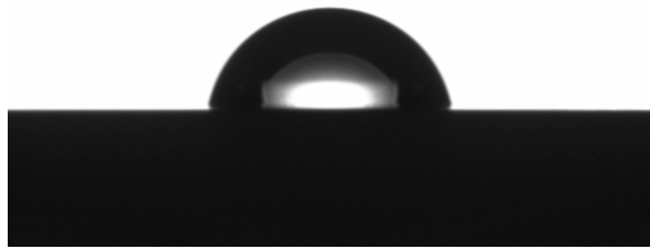
Figure 73. Representative water droplet image on copper
