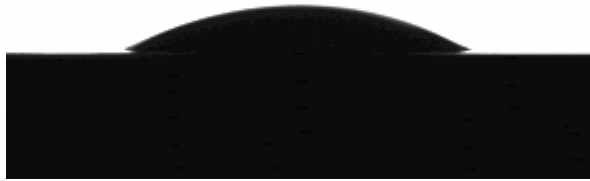
Figure 74. Representative water droplet image on solder mask
