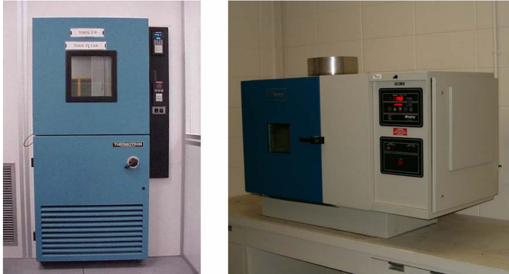
Figure 15. Humidity chambers used for moisture preconditioning test specimens
