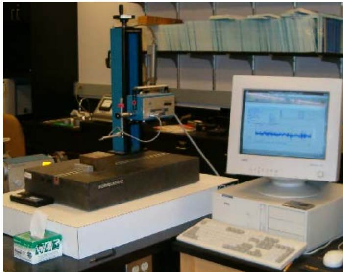
Figure 19. Profilometer used to measure surface roughness
