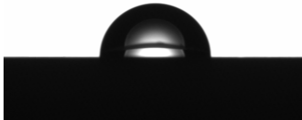
Figure 75. Representative water droplet image on underfill
