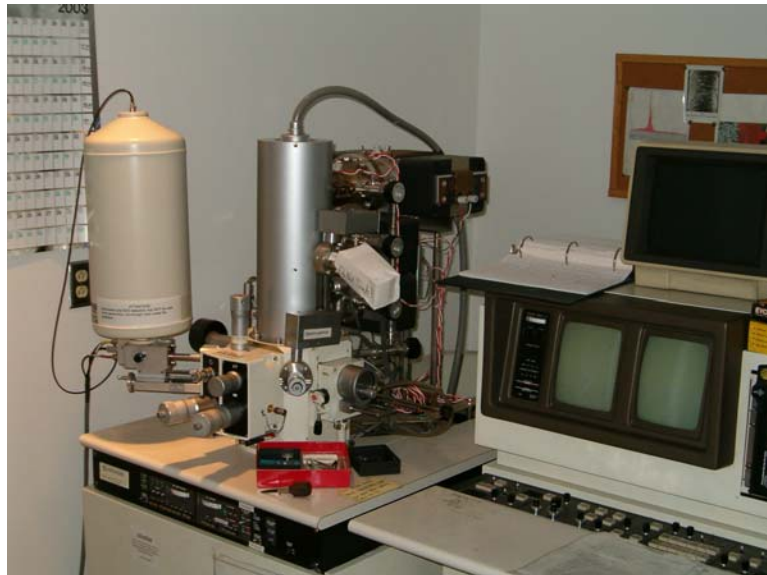
Figure 21. Scanning Electron Microscope used to examine fracture surfaces
