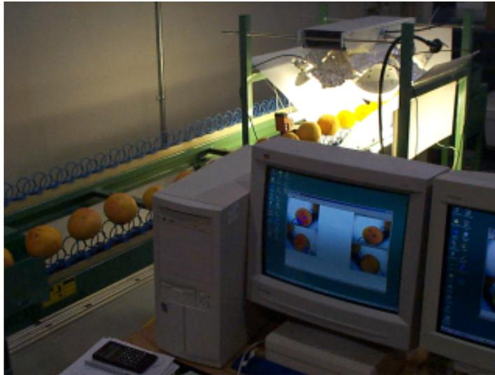
Figure 5.19: Picture showing lab prototype of the grapefruit inspection cell
