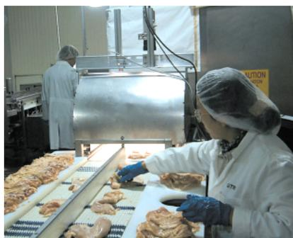
Figure 5.15: Prototype fan bone detection system online at input to X-Ray imaging system
