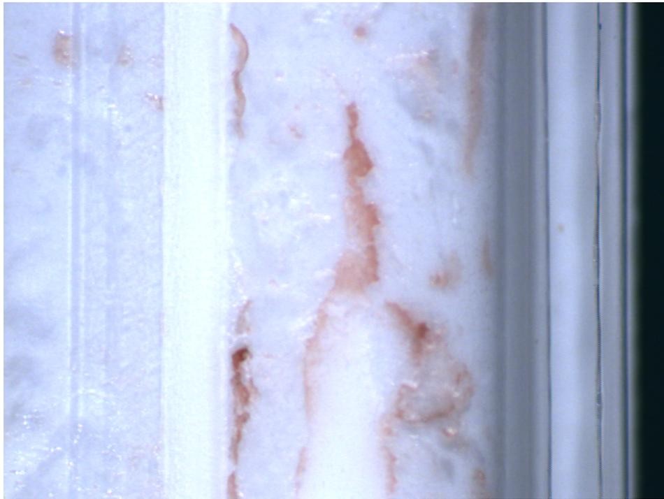
Figure 5.26: Package seal with contamination
