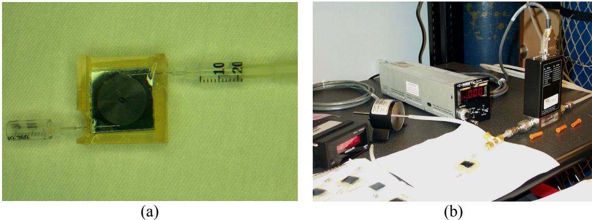
Figure 7-1. Experimental setup for the flow test of a parylene column (a) prepared sample, (b) flow test setup.
