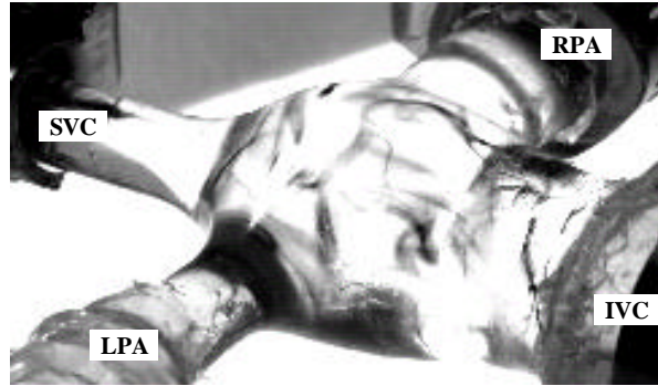
Figure 6.2.13: Model 6. Qualitative flow visualization at 1L/min and with a pulmonary flow split of 70/30 RPA/LPA seen from the side. The recirculation region occupied the entire connection region, leading to important 3D mixing of the caval flows.
