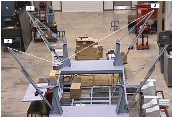
(a) Prototype of the Cable Array Robot.
