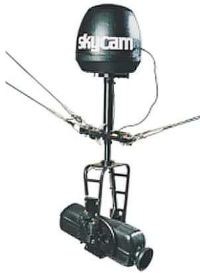
(a) A closeup of the SkyCam end-effector [26].
