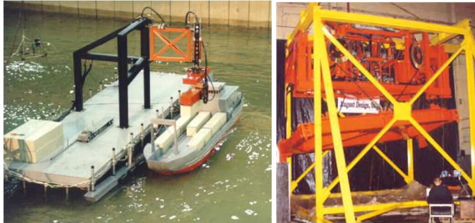
(a) The AACTS unloading cargo from a ship [6].
