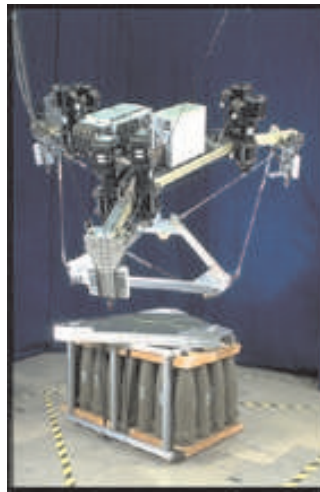
(c) The ROBOCRANE modified to handle munitions.
