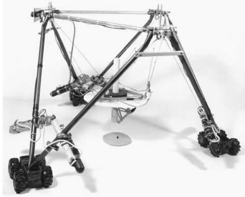
(a) A scale model of the ROBOCRANE mounted to mobile bases.
