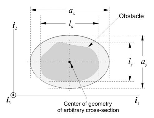
Figure 34: Enveloping the arbitrary cross-section in an ellipse
