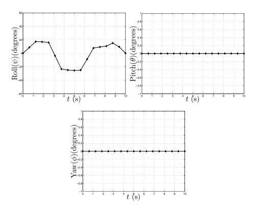
Figure 40: Inertial orientations for vertical cylinder avoidance case
