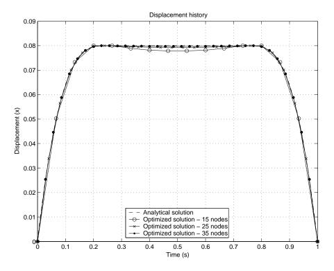
Figure 17: Optimized displacement and analytical solution
