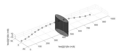
Figure 39: Feasible vehicle trajectory avoiding vertical cylindrical obstacle
