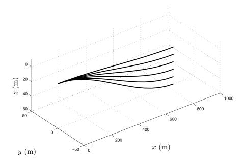
Figure 24: Family of dives with increasing final depth.
