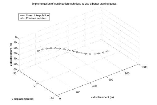
**Figure 22:** Application of continuation technique to arrive at dive of 60 m using a better starting guess (i.e. solution to 50 m dive problem).
