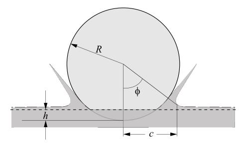
Figure 14: Immersion of the cylindrical profile in water.
