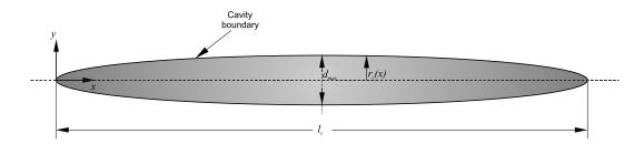
Figure 7: Cavity dimensions calculated using Reichardt formulation.
