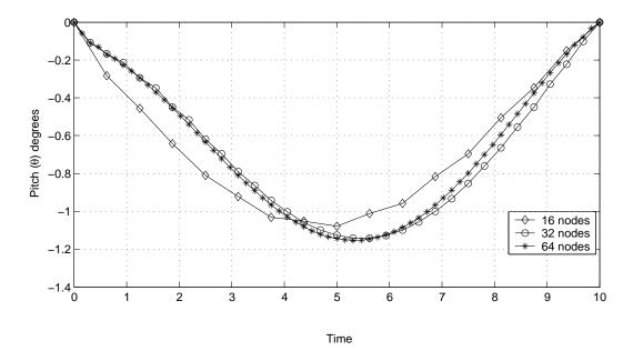
Figure 21: Convergence of solution as a result of bootstrap technique.
