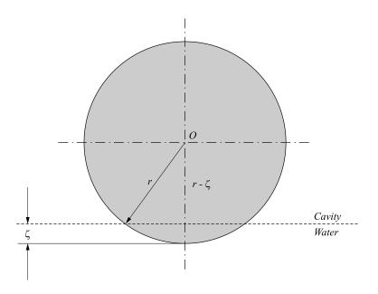
Figure 13: Partly immersed tail section.
