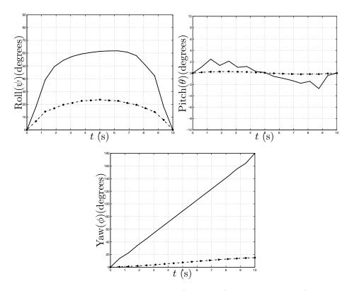
Figure 29: Inertial orientations for  $60^{\circ}$  (solid line) and  $180^{\circ}$  turns (dashed line)
