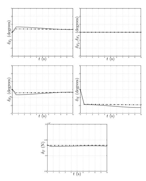
**Figure 31:** Control time history for 10 m (dashed line) and 60 m dives (solid line) for control velocity minimization case.
