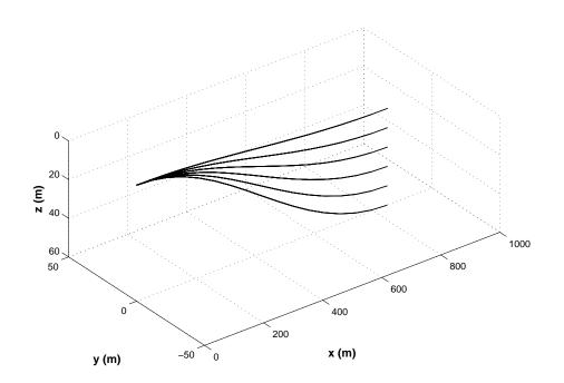
**Figure 30:** Vehicle trajectories for a family of dives with control velocity as the objective function
