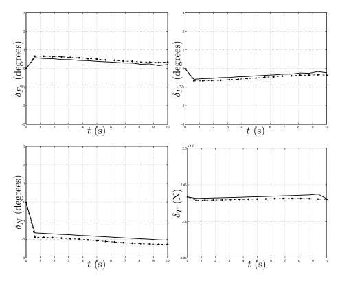
**Figure 33:** Control time history for 60 m dives with control velocity minimization (dashed line) and control effort minimization (solid line)
