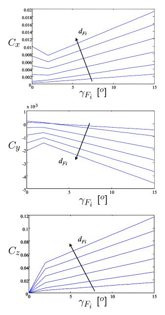
Figure 10: Fin force coefficients versus angle of attack, for varying penetration depth.
