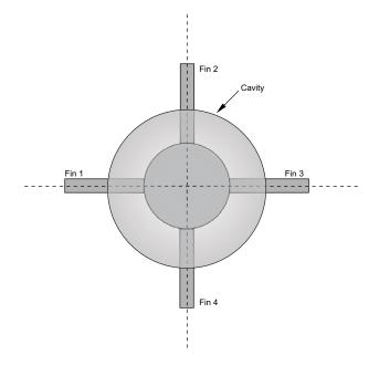
Figure 5: View of cruciform arrangement of fins (view from behind the vehicle)
