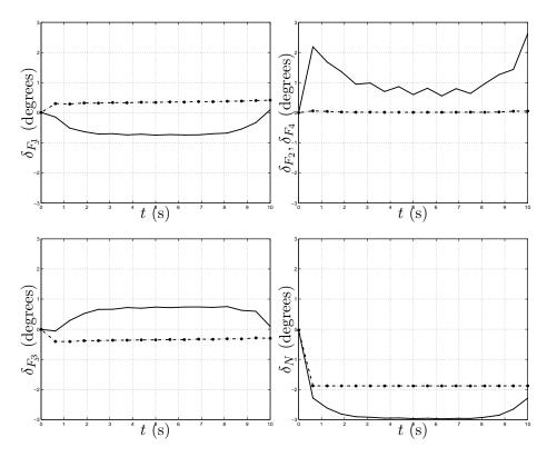
Figure 28: Control time history for  $60^{\circ}$  (dashed line) and  $180^{\circ}$  turns (solid line)
