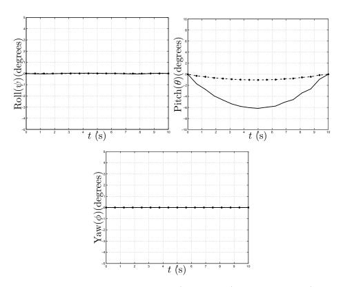
Figure 26: Inertial orientations for 10 m (dashed line) and 60 m dives (solid line).
