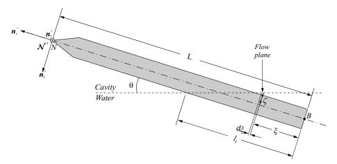
Figure 12: Impact force and moment calculation.
