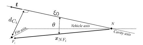
Figure 11: Calculation of fin penetration depth.
