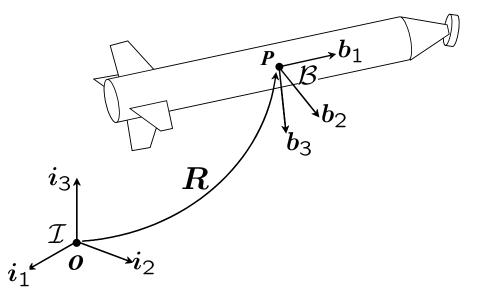
Figure 6: Body-fixed and inertial frames.
