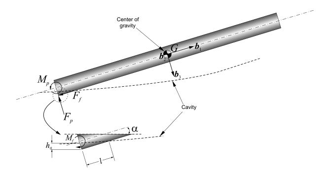
Figure 15: Planing of the cylinder on the cavity surface.
