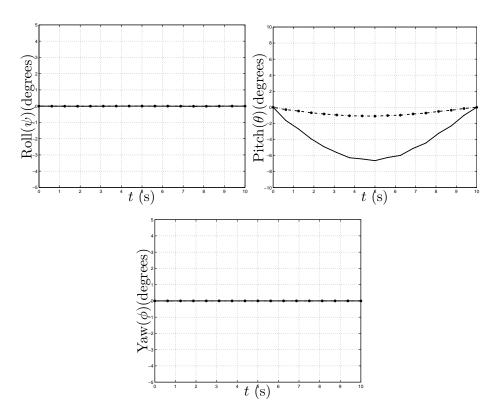
**Figure 32:** Inertial orientations for 10 m (dashed line) and 60 m dives (solid line) for control velocity minimization case
