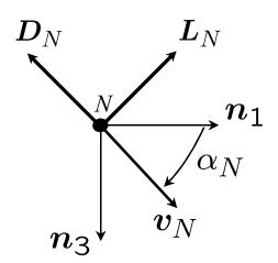
(a) Lift and drag components in the  $\boldsymbol{v}_N$ ,  $\boldsymbol{n}_1$  plane.
