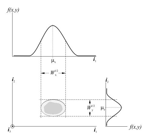
Figure 36: Using the Gaussian function to assign trajectory constraint violation
