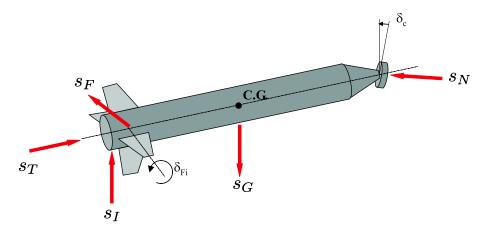
Figure 4: Configuration of supercavitating vehicle with applied forces.
