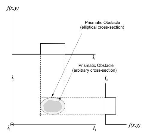
Figure 35: Using a step-function to assign trajectory constraint violation
