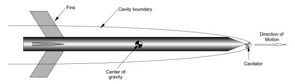
Figure 3: Configuration of the supercavitating vehicle.
