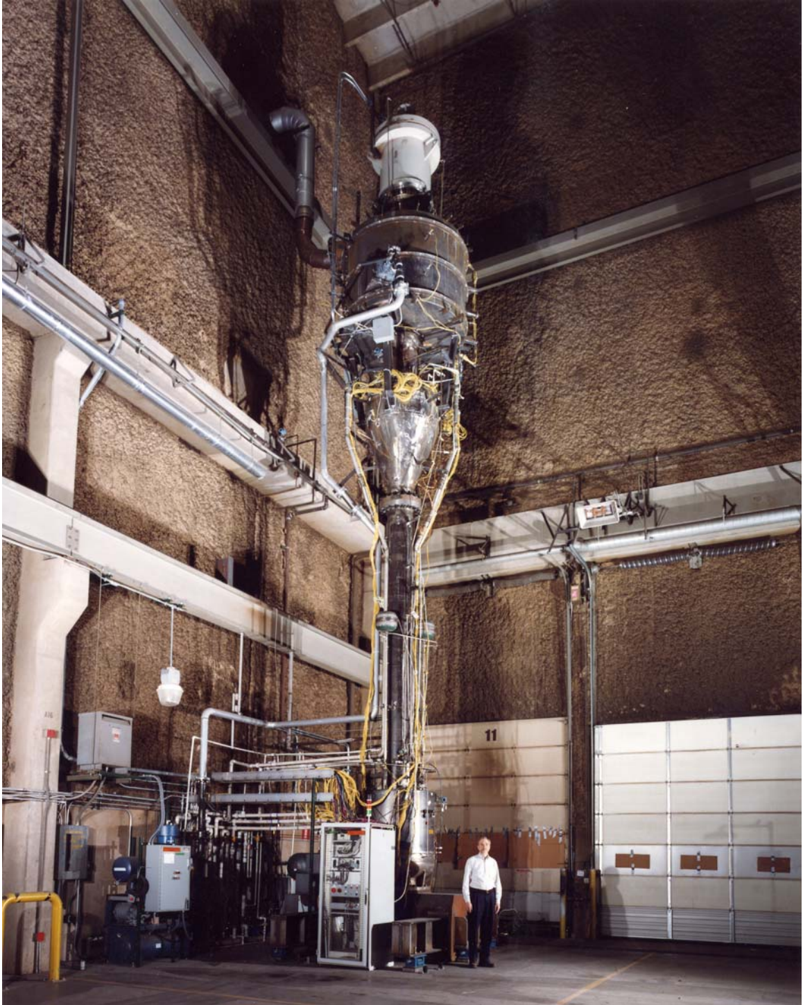
Figure 3.6: The 350 gallon per day natural gas liquefier. (Photo courtesy of Greg Swift)
