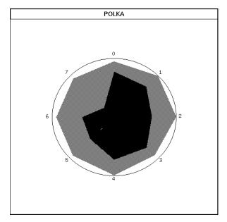
Figure 7: Kiviat diagram, created using POLKA, that shows average processor utilization over a given time interval.
