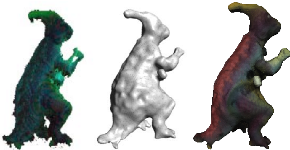
Fig. 18. From left to right: volumetric data set of the toy dinosaur from space carving, reconstructed implicit surface generated using the multi-order basis, reconstructed implicit surface textured using the original images.
