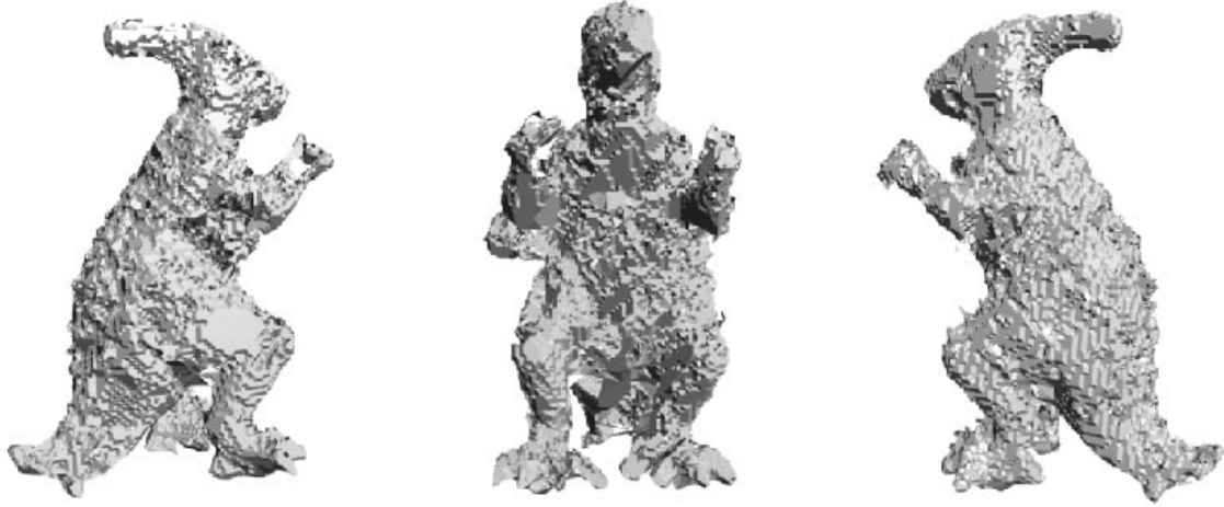
Fig. 1. The data set is a space carved volume of a toy dinosaur. The reconstruction was obtained from the Crust algorithm.
