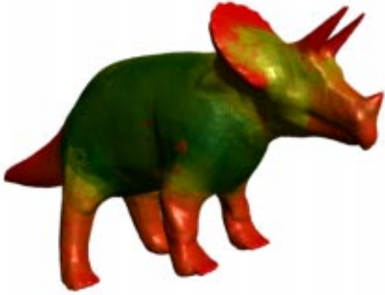
Figure 3: This figure illustrates the radius of regularity. Thin regions such as the dinosaur’s collar and high-curvature regions such as the tips of the horns have a smaller radius and are colored red, and lower curvature regions are more green.
