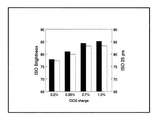
Figure 4. Chlorine dioxide brightening of L(EOP)LE pulp with different  $ClO_2$  charges. Solid bar is ISO brightness, and open bar is ISO brightness after thermal reversion equal to 25 years.
