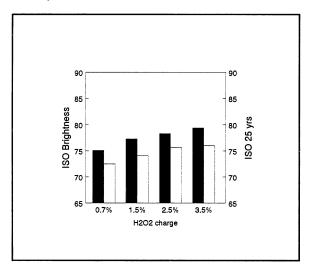
Figure 3. Hydrogen peroxide brightening of L(EOP)LE pulp with different  $H_2O_2$  charges. Solid bar is ISO brightness, and open bar is ISO brightness after thermal reversion equal to 25 years.
