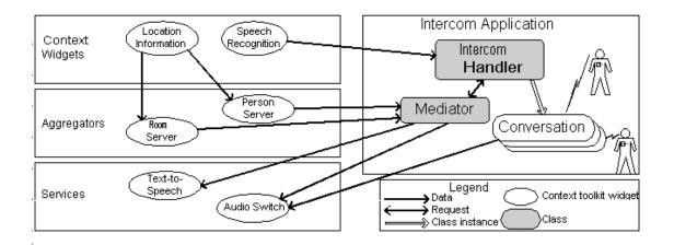
Figure 2 - IntercomApplication Software Design
