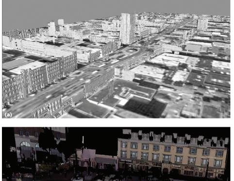
1 (a) Overview of Berkeley, California, facade mesh. (b) Detail from mesh with textures. (Courtesy of Avideh Zakhor.)
