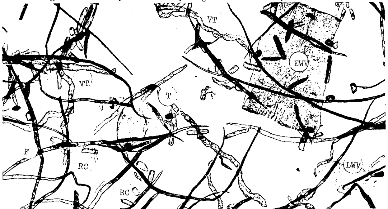
Figure 9. Pulp Sample of Red Oak Bleached Kraft (Submitted by Hammermill Paper Co.). Earlywood Vessel Element (EWV), Latewood Vessel Element (LWV), Tylosis (T), Fibers (F), Vasicentric Tracheids (VT), Ray Cells (RC). Magnification - 90 Diameters, Weight Factor - 0.48. Note: Tyloses are not Common in Species of Red Oak. The Pulp Sample is Possibly Contaminated with a Percentage of White Oak
