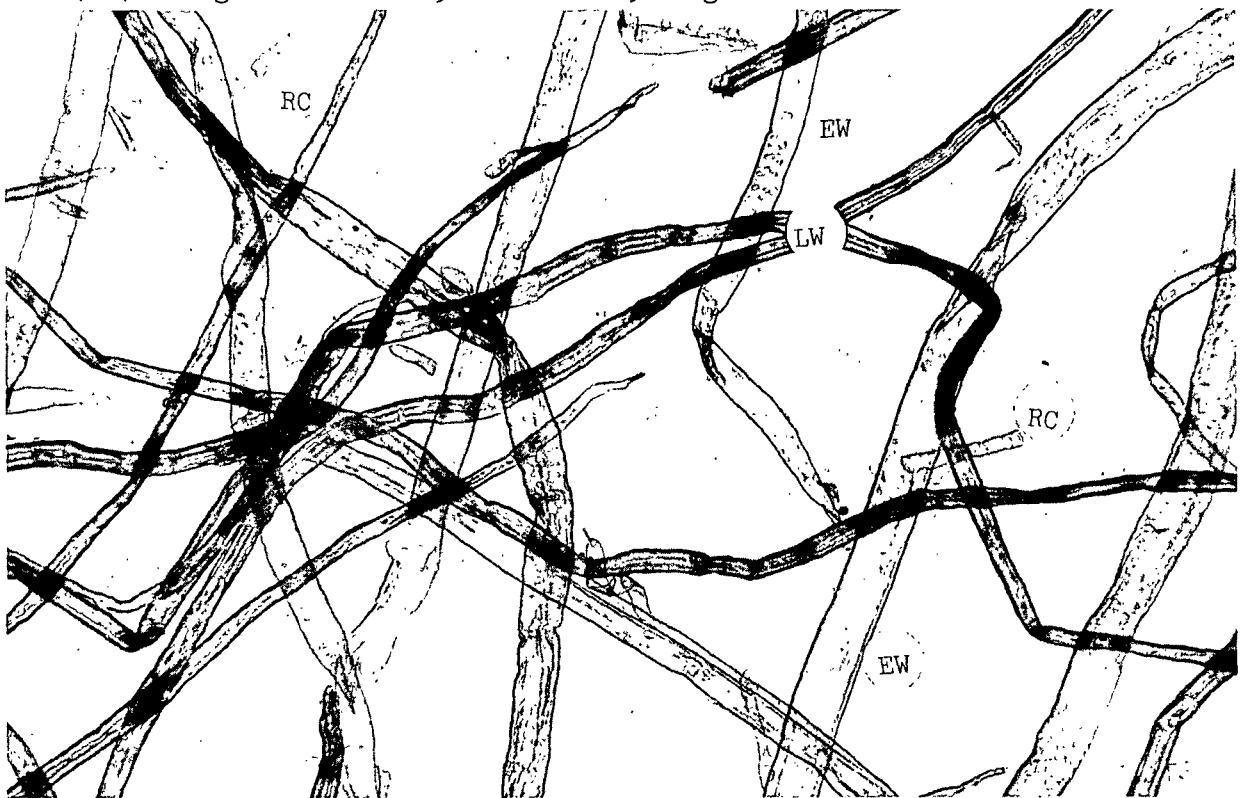
Figure 4. Pulp Sample of Loblolly Pine Bleached Kraft (Submitted by Hammermill Paper Co.). Latewood Tracheids (LW), Earlywood Tracheids (EW), Ray Cells (RC). Magnification - 90 Diameters, Weight Factor - 1.25
