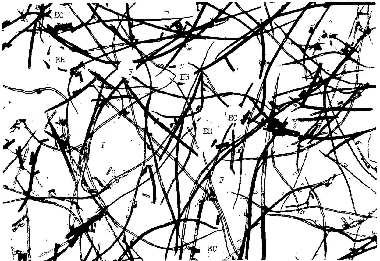
Figure 14. Pulp Sample of Esparto Bleached Kraft-Tunisia (Submitted by Riegel Paper Corp.). Fibers (F), Epidermal Cell (EC) with Scalloped Wall, Epidermal Hairs (EH). Magnification - 90 Diameters, Weight Factor - 0.43
