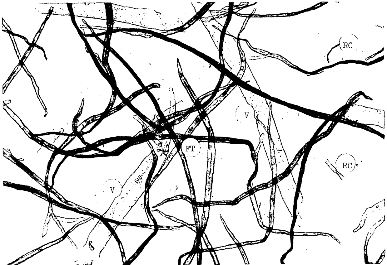
Figure 7. Pulp Sample of Sweetgum Bleached Kraft (Submitted by Hammermill Paper Co.). Fiber Tracheids (FT), Vessel Elements (V), Ray Cells (RC). Magnification - 90 Diameters, Weight Factor - 0.84
