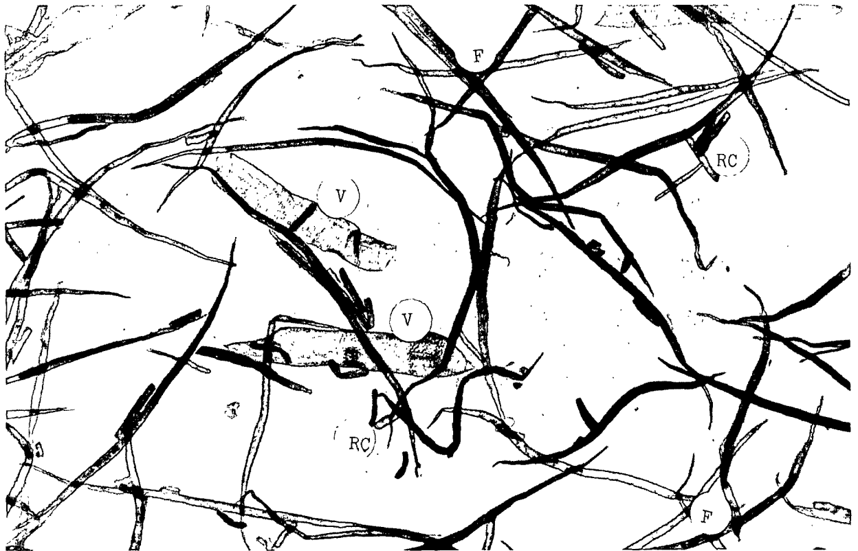
Figure 10. Pulp Sample of Maple Unbleached Kraft (Submitted by Hammermill Paper Co.). Vessel Elements (V), Fibers (F), Ray Cells (RC). Magnification 90 Diameters, Weight Factor - 0.37
