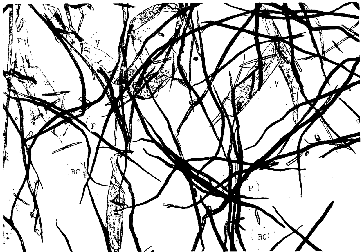
Figure 12. Pulp Sample of Beech Unbleached Kraft (Submitted by Scott Paper Co.). Vessel Elements (V), Fibers (F), Ray Cells (RC). Magnification - 90 Diameters, Weight Factor - 0.50
