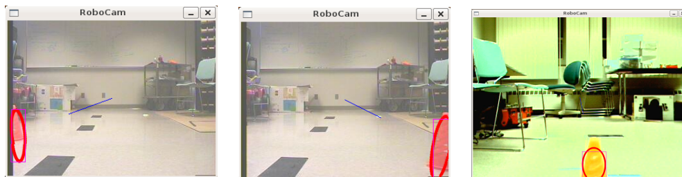
(a) The cone is too far left of the robot (b) The cone is too far right of the robot (c) The cone is too close to the robot
