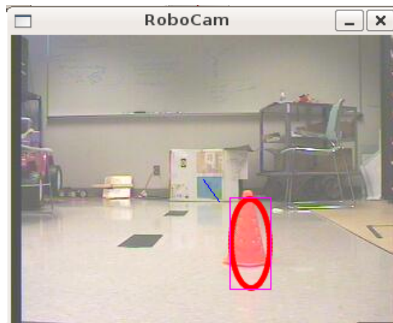
Figure 25: A frame from the lab environment with the cone 150 centimeters away from the Pioneer 2 robot
