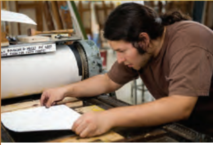
Javier Rodriguez '08 uses a Vandercook press to print a linoleum block.
