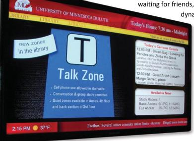
updated over the internet. The UMD Library runs their system on an in-house Linux server using the free open source Xibo (pronounced eX-E-bO) client/server solution. The visuals are designed in Photoshop, with animations done via Powerpoint. The wall-mounted 52" LCD TV is an effective way to reach a lot of people in a high-traffic area and has been great for promoting library and campus-wide services and events.
