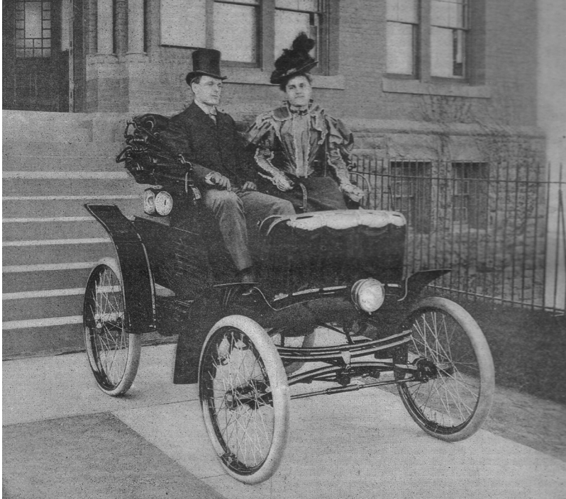
FIG. 2 An 1897 Columbia electric horseless carriage, built by the Pope Manufacturing Company (bestseller during 1897–98). (Source: Scientific American , 22 May 1897, 331.)
