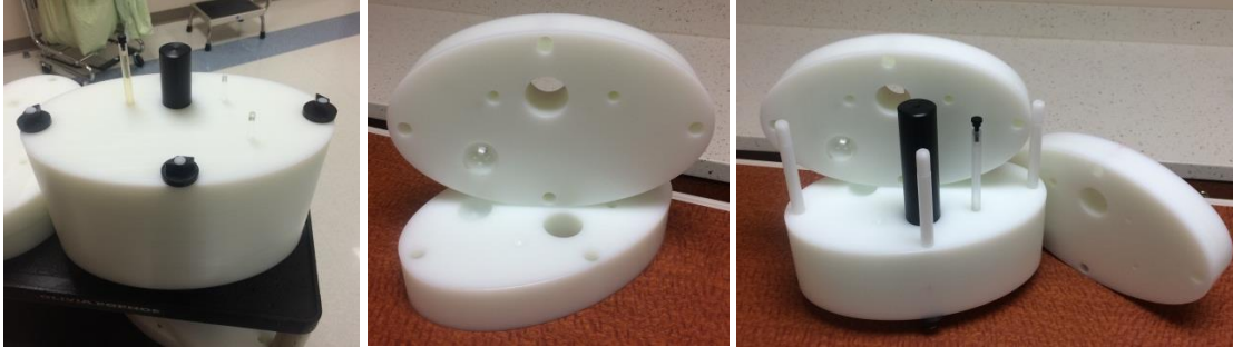
Figure 5. Custom designed small phantom fully assembled (left image), the center two plates (center image), and half assembled (right image)
