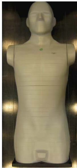
Figure 2-5 – Anthropomorphic phantom - Photograph of the anthropomorphic phantom used for the TLD measurements the prescribed dose.
